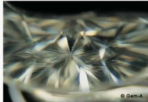
Strong doubling seen in synthetic moissanite © Gem-A
